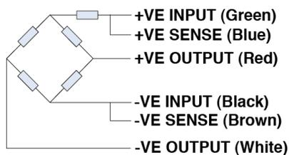
**WIRING SCHEMATIC DIAGRAM (1015)**
