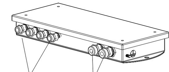
4x M12, a.f. 14 for cable diameter 5 ... 6.5 mm
