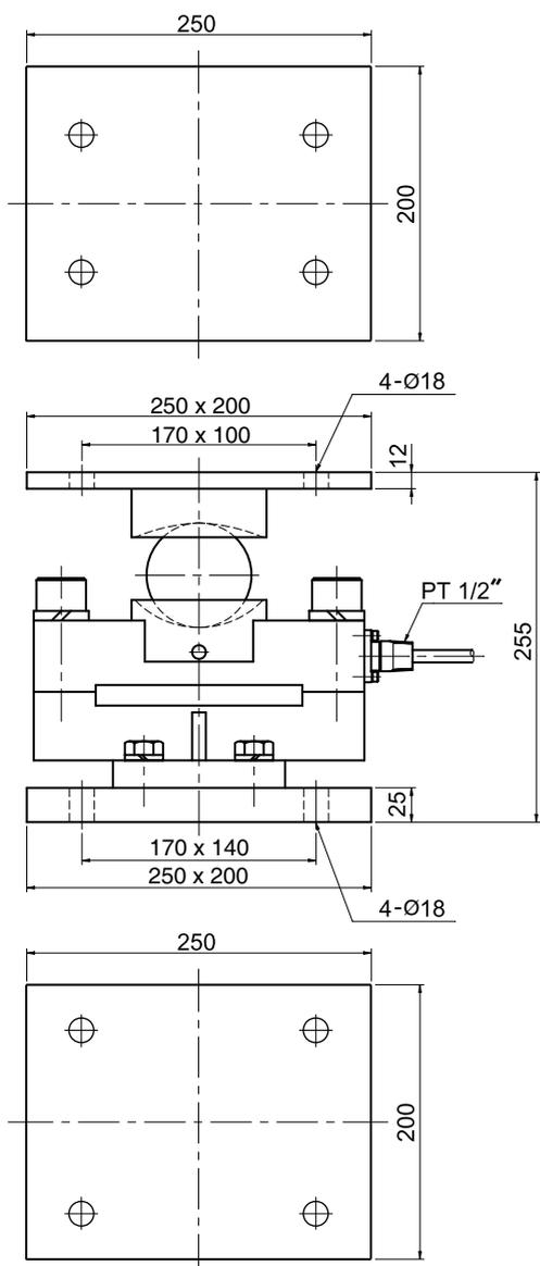
The model of CDUP is specially designed for truck and railroad scales in harsh environments. The effective integration of the CDUP mount and double ended shear beam load cell eliminates the need for troublesome check roads, links, expansion assemblies and other peripheral hardware.
