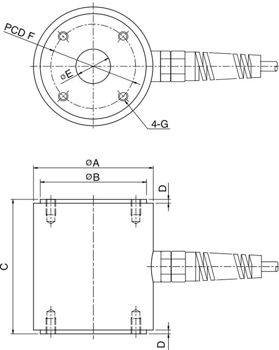
The BCH series is designed for the load control and the monitoring during the power inserting using the press. It is also designed user-friendly; each 4 threaded holes, on top and bottom, with the flange type are very helpful while the installation.
